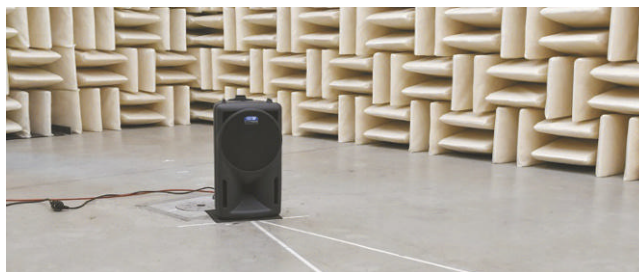
Test set-up for the M-Noise test in the measuring lab's anechoic chamber. In front: The 1/4" B&K 4939 measurement microphone with impedance converter
